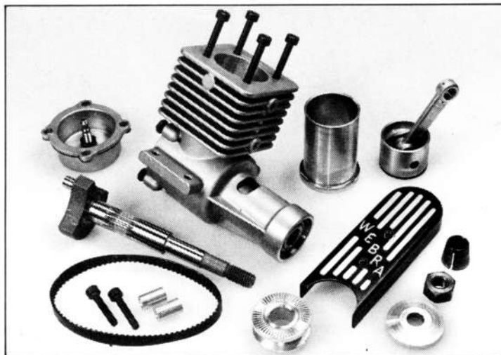
Parts of T4-40. Engine features Dykes-ringed piston running in chromed brass sleeve. Note splines on crank for toothed belt drive.
